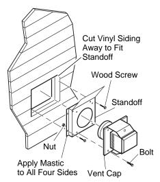
Figure 14 - Installing Vinyl Siding Standoff
